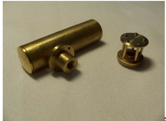
olid brass end cap / manifolds to hollow exhaust uprights
